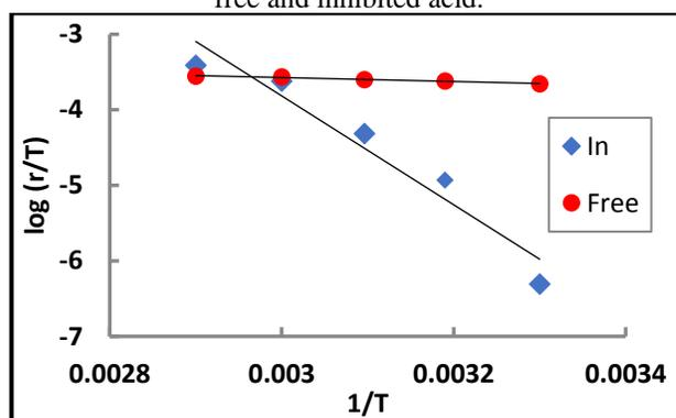
Fig (8): Transition state plots for corrosion of aluminum alloy in free and inhibited acid.
