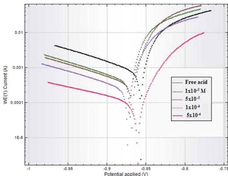
Fig (3): polarization curves for aluminum-silicon alloy in free and inhibited 2 M HCl solutions.
