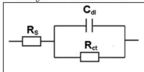
Fig (5): Randles equivalent circuit.
