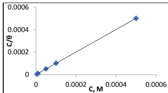
Fig (6): Langmuir adsorption isotherm
