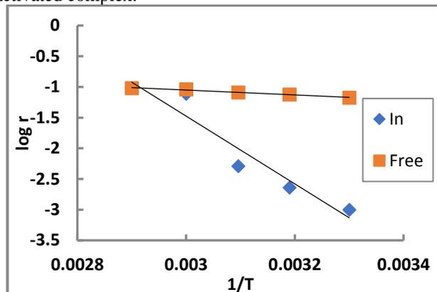
Fig (7): Arrhenius plots for corrosion of aluminum alloy in free and inhibited acid.
