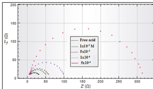
Fig (4): Nyquist diagram obtained for the alloy in free and increasing concentrations of caffeic acid.
